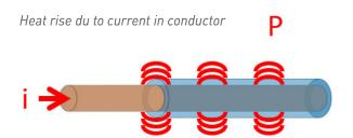
Heat rise due to current in the conductor is  $P = R \times i^2$
