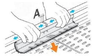
Keep a gap "A" between two tray lengths as indicated on coupler
