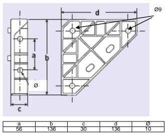
To fix pendant channels with ceiling brackets, use the nut and bolts M8x20
