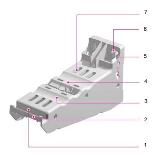
1- Hook for attaching cover during maintenance
