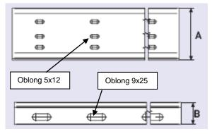
Slots 9x25mm in base of divider allow fixing with M8 screws
