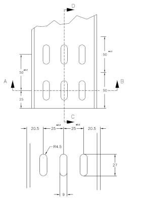
To fix pendant channels with ceiling brackets, use the nut and bolts  $\ensuremath{\mathsf{M8x20}}$
