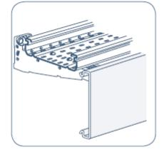
For easier installation, the cover can be simply hooked on the bracket during maintenance operations
