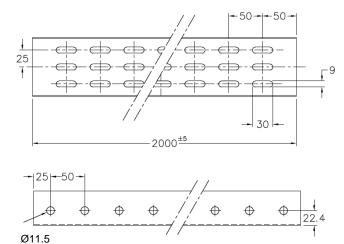
To fix pendant channels with ceiling brackets, use the nut and bolts M8x20
