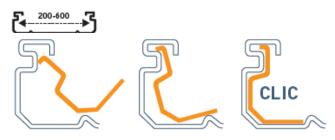
Marking system for installing couplers according to temperature conditions (20, 40 or  $60^{\circ}$ C) to enable the PVC to expand.
