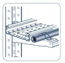
Special holes have been designed for fitting clamps so that pipes can be fixed on the bracket
