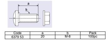
For fixation of profiles without load bearing applications.
